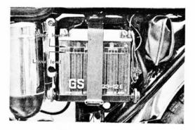
Check to see that the overflow tube is not clogged.
