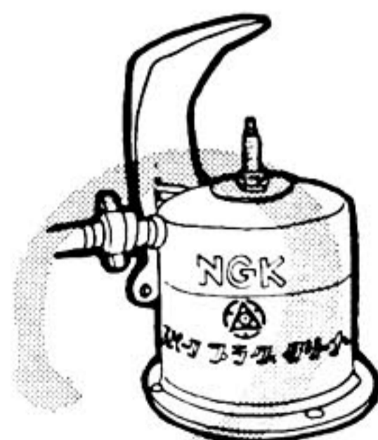
It is the best way to clean a plug with the NGK plug cleaner.
